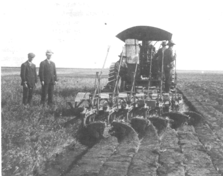
Fig. 19. Breaking sod with a Hart-Parr tractor and six-bottom gang plough. Asquith District, Saskatchewan, ca. 1910. This outfit was very similar to W.R. Motherwell's tractor and gang plough. (Saskatchewan Archives Board, Regina, R-A12, 082).
