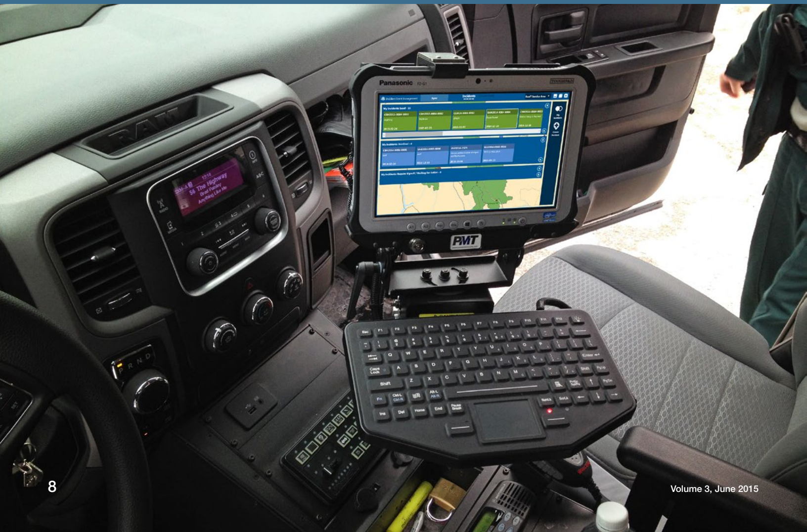
Figure 9: The Incident and Event Management (IEM) System is a map-based system that runs on mobile tablets that are carried by National Park Wardens or mounted in their vehicles. IEM continues to function while disconnected from the PCA network and cellular signals. Upon returning to the office, the system synchronizes any changes with the central database. (Simulated screen content for illustrative purposes).
