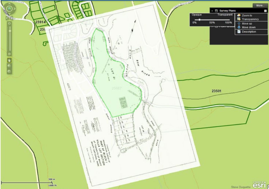
Figure 7: This screen-capture from NIRS shows how Realty staff can “rubber-sheet” a survey plan to the base-map so the plan can be more easily found, understood, and related to other map information. A transparency slider allows the user to fade the survey in and out of the foreground.
