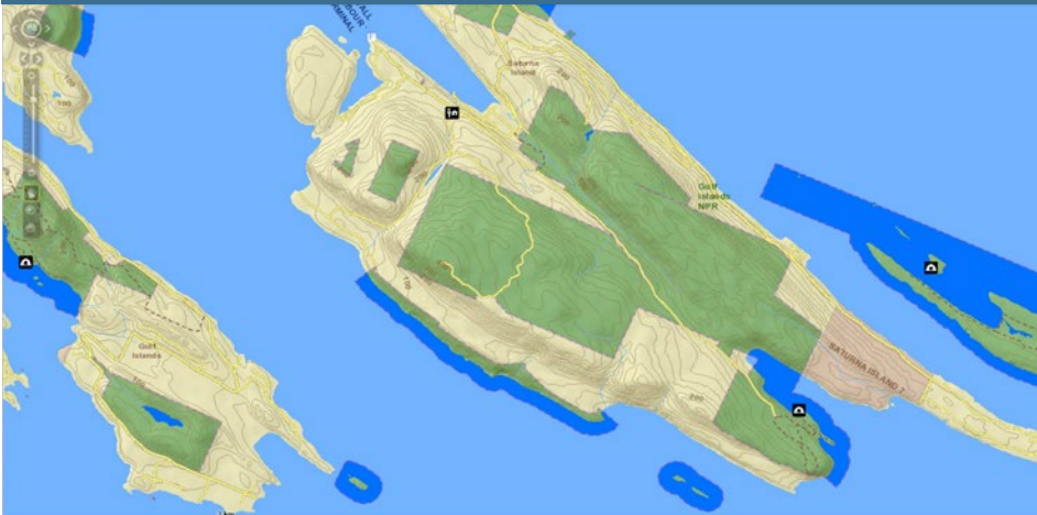
Figure 2: Example map from the Parks Canada Geomatics Infrastructure. Maps like this one (at 1:36,000 scale) are available for all of Canada. Note how the map is tuned to the business requirements of Parks Canada. Green areas are national park lands, darker blue is national park waters, and pink areas are Indian Reserves. The icons represent a Parks Canada office and campgrounds.
