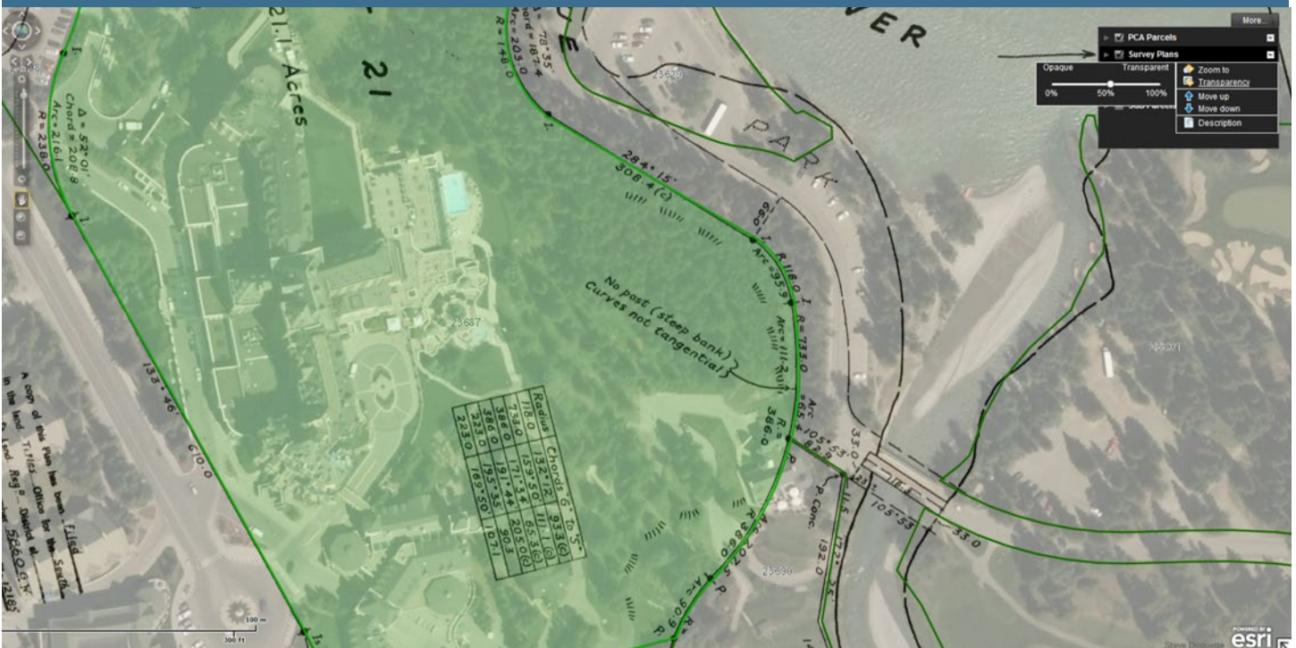
Figure 8: Close-up view from NIRS showing the survey plan superimposed on the air-photo. This type of view helps Parks Canada managers relate the survey (and therefore the lease agreement) to features on the ground.
