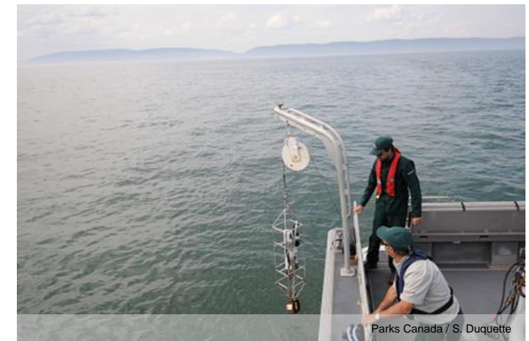
CTD type probe deployment to measure temperature, salinity and dissolved oxygen through the water column
