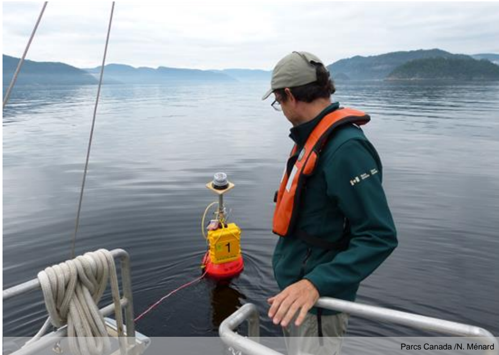
Deployment of a drifting buoy with hydrophones to measure sound propagation in the Saguenay Fjord
