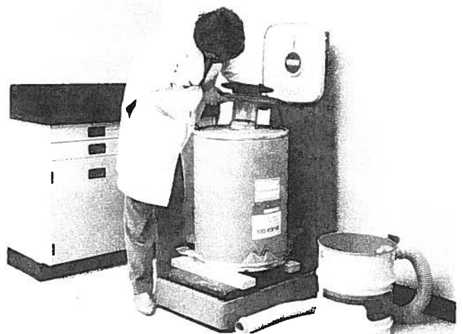
Figure 15: The drum is inverted and placed over spacers. In what was originally the bottom of the drum, a hole is cut to the size of the blower section of a wet-dry vacuum cleaner. The blower section is then inserted into this hole and seams are well sealed.
