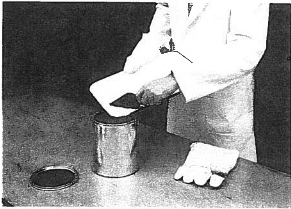
Figure 8: Hot silica gel is placed in a metal container which is then sealed.
