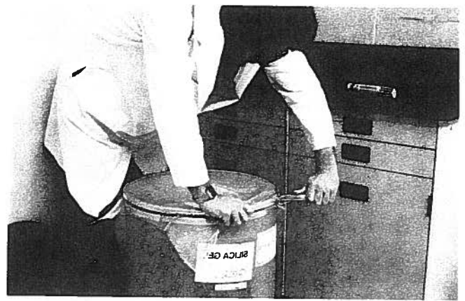
Figure 14: The cover is replaced with aluminum screening which is held in place by the original retaining ring.
