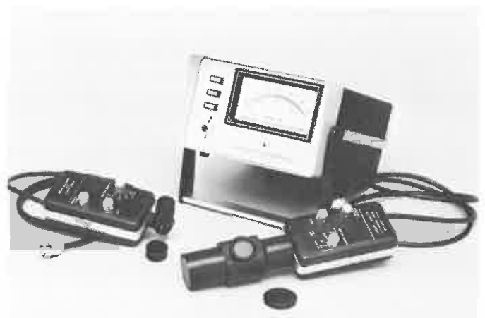
FIGURE 13. Gamma Scientific Model 900. Left detector head measures illumination; the other measures UV intensity from 300nm to 400nm.
