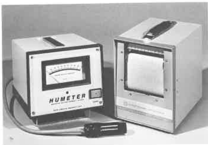
FIGURE 4. Some electronic hygrometers have an output for connecting a strip chart recorder to give continuous readings. The "Humeter" uses a separate sensor.
