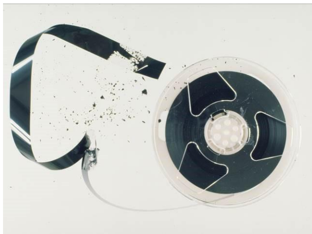
Figure 7. Flaking of binder and magnetic particles from the base of a VHS tape. This may be due to binder degradation or failure of the adhesion between binder and base for other reasons.
