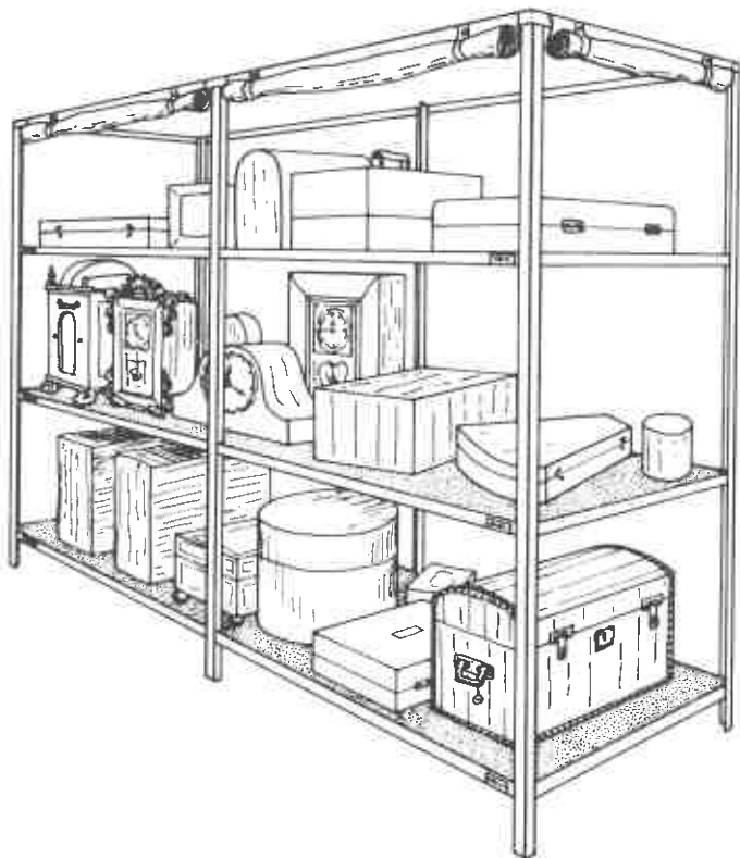
Figure 6: Ideal storage shelves for medium size objects. Note the top shelf is not used for storage; it is there to protect artifacts. Also, the lower shelf is raised off the floor if the shelves are located in the basement. Dust flaps are shown rolled up in this illustration.
