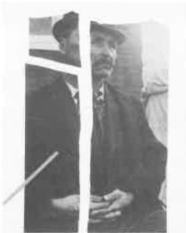
Figure 46: This brittle, unmounted print, broken into a number of pieces, has a fracture (adjacent to the pointer) and has completely lost one area.
