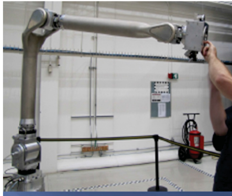
Figure 9: Active support: robotic arm (Bailey, 2013). (source: DRDC)
