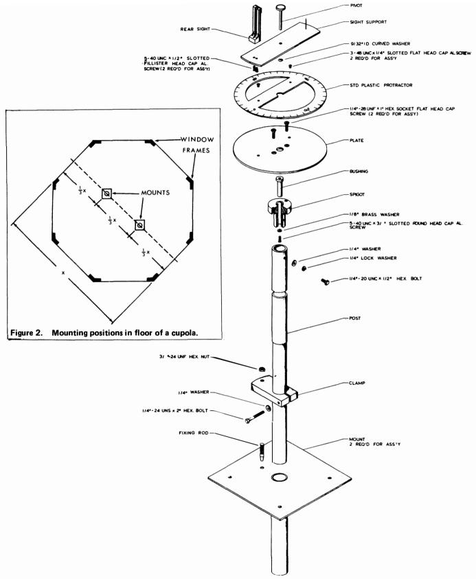
Figure 1. Schematic illustration of the NoFRC firefinder.
