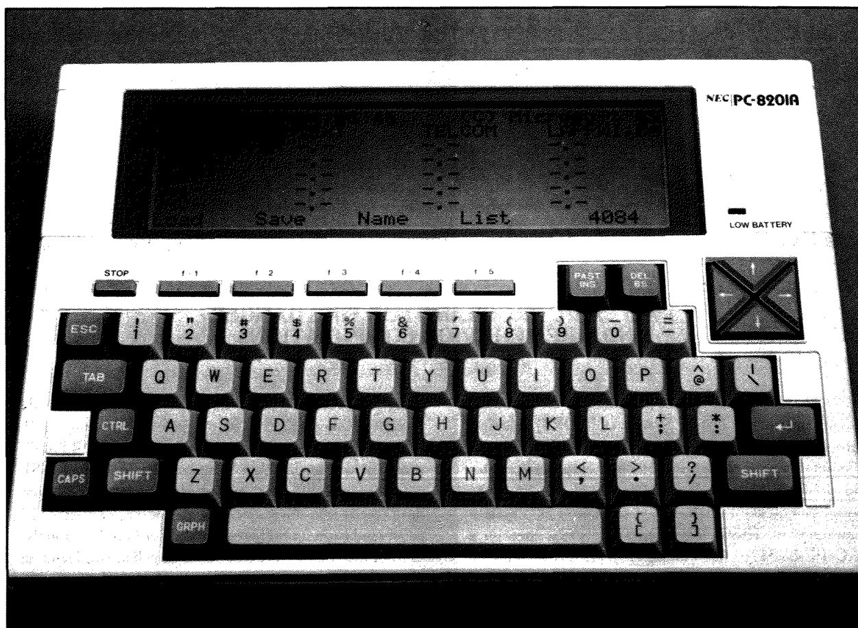
Figure 1. The NEC PC8201A lap computer measures 30 \times 21 \times 3.5 cm and weighs 1.7 kg.
