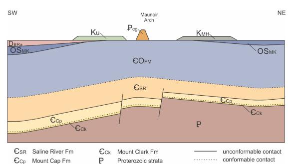
Figure 2. Schematic stratigraphic relationship diagram for the Lac Maunoir map area (NTS 96-N). Subsurface relationships are based on public-domain reflection-seismic data and petroleum exploration wells.
