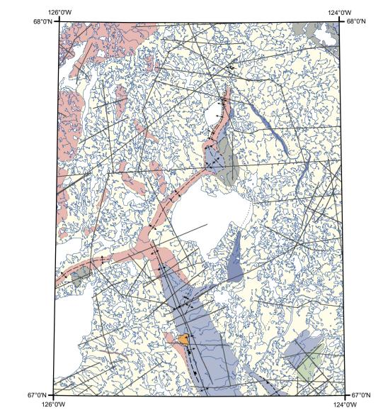
Figure 1. Lac Maunoir map area (NTS 96-N) showing seismic lines (grey lines) on record with the National Energy Board (NEB) that were used to augment the bedrock geology interpretation. Line names are provided in the digital
