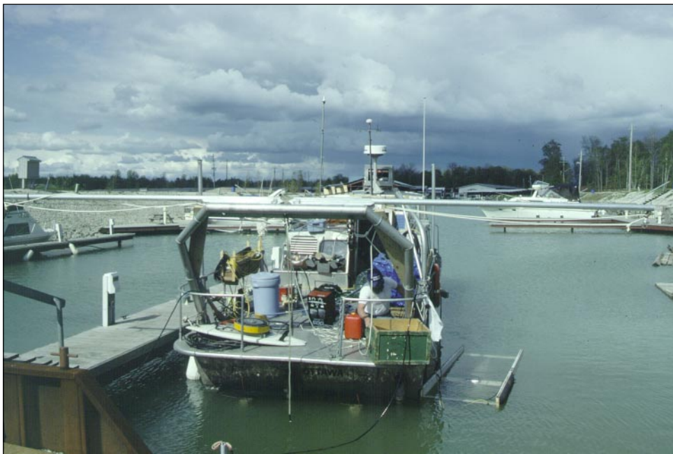
20. The MV J. Ross Mackay at Big Bay Point Marina, Lake Simcoe, May, 1993. The Seistec system is in the water for testing. The booms are extended off the A-frame for outfitting.
