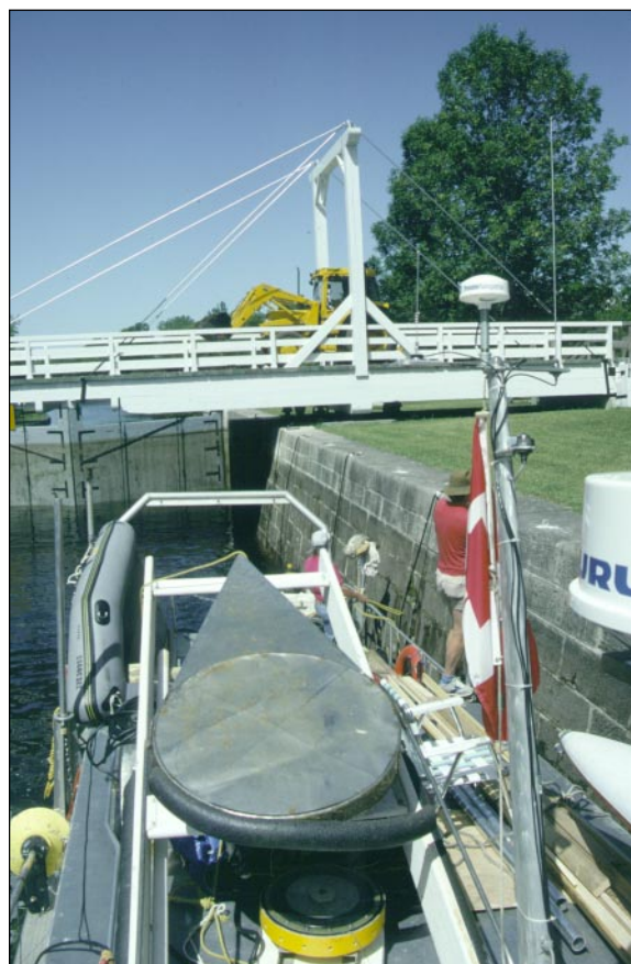
3. The ship in a lock on the Rideau Canal, 1992. The upturned Seistec receiver cone is in the foreground, straddling the Seistec boomer mounted on a surfboard.
