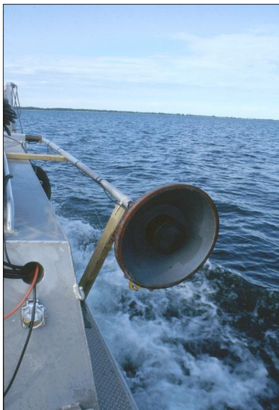
1. 3.5 kHz sounder mounted on the starboard side.
