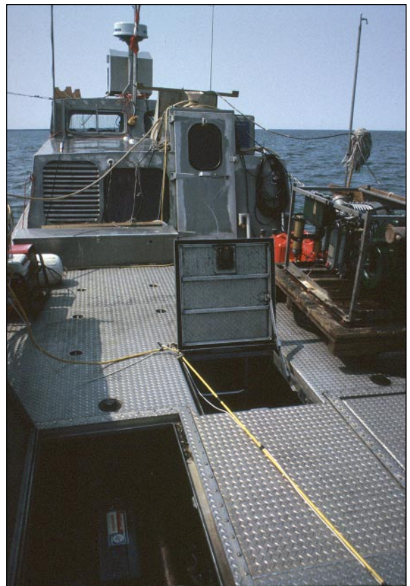
24. Deck configuration of the MV J. Ross Mackay while towing survey instruments. Hatches to the diesel engines are open to allow heat to escape. Door to the laboratory is closed due to the high noise level on deck.
