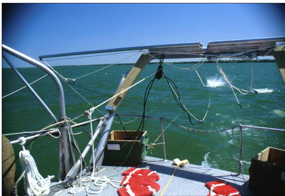
2. Sunny day surveying on Lake Simcoe. Note that the IKB Seistec surfboard (far right) has been adjusted to tow below the water surface. This configuration reduced the amount of noise on the records.
