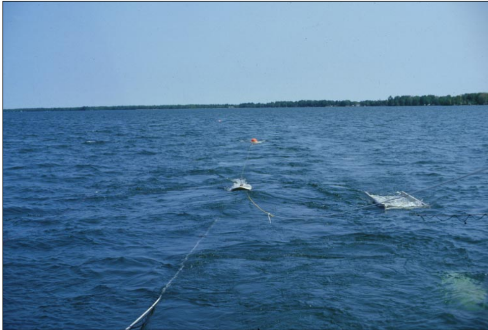
23. Towing survey instruments. The beginning and end of the seismic eel are denoted by the orange floats in the distance. Note seismic boomer surfboard towing beneath the water surface on the lower right.
