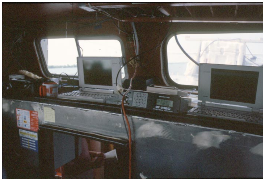
10. Wheel-house of the MV J. Ross Mackay showing the computer setup for recording GPS navigation and magnetics.
