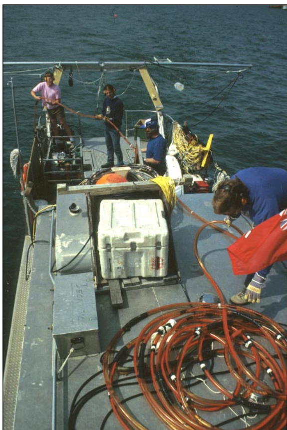
19. Paying out the oil-filled seismic eel over the starboard stern. From left to right are Marten Douma, Paul White, Robert Burns and Brian Todd.
