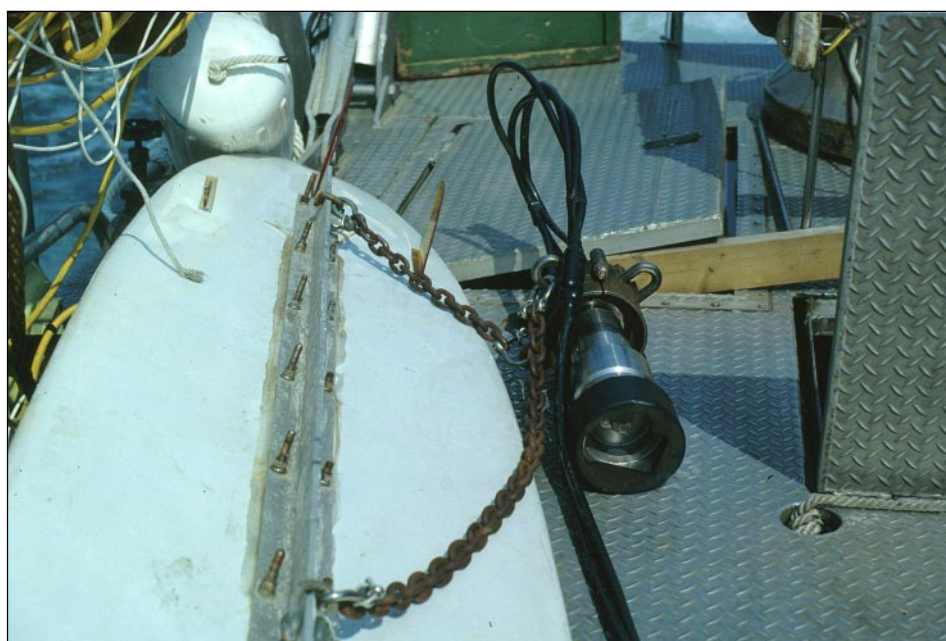
6. Close-up of surfboard with airgun attachment.
