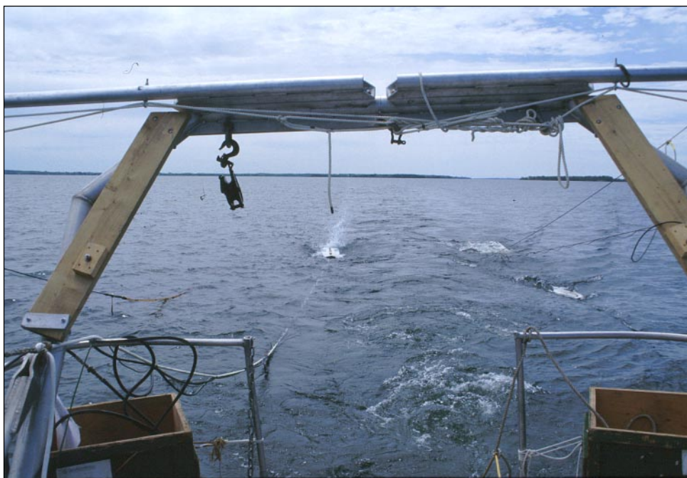
1. View aft of the ship showing the instrument towing arrangement. In the centre of the image is the surfboard under which the airgun multichannel seismic source is slung. On the right is the IKB Seistec receiver (aft) and the surfboard (forward) under which the Seistec boomer source is slung.
