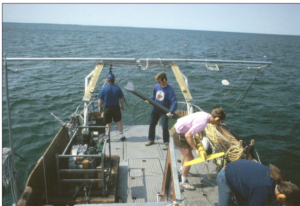
20. Launching the magnetometer towfish (dark grey) and sidescan sonar towfish (yellow). From left to right are Robert Burns, Brian Todd, Marten Douma and Paul White. The beginning and end of the seismic eel are denoted by the orange floats in the distance.
