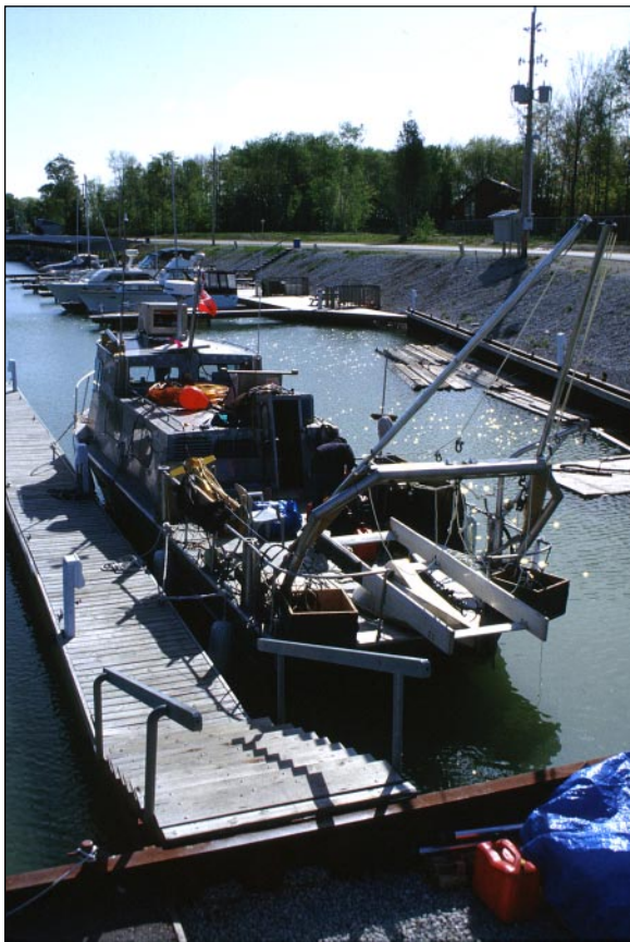
2. MV J. Ross Mackay at Big Bay Point Marina, Lake Simcoe. The IKB Seistec receiver is secured over the stern for travel to the start of the survey line.
