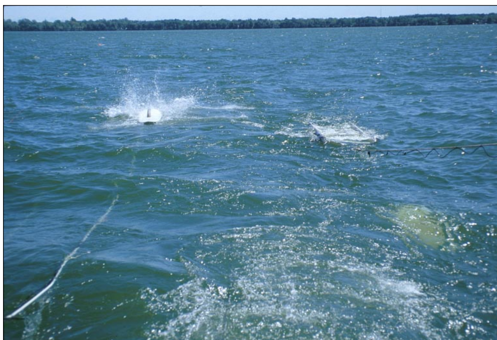
4. Survey tow arrangement. Note IKB Seistec boomer surboard (lower right) below water surface.
