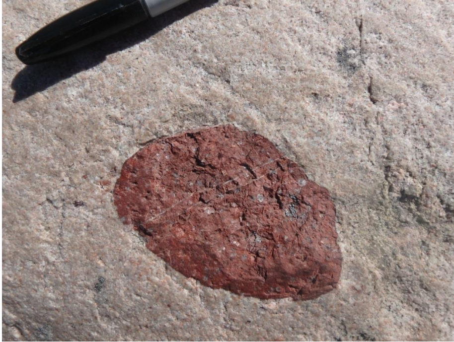
Figure 14: Outcrop photograph of massive, conglomeratic arkose on Porter domain basement. Isolated rounded clasts of red, trydimite-phyric rhyolite occur within pink arkosic arenite. Field of view is 15 cm.
