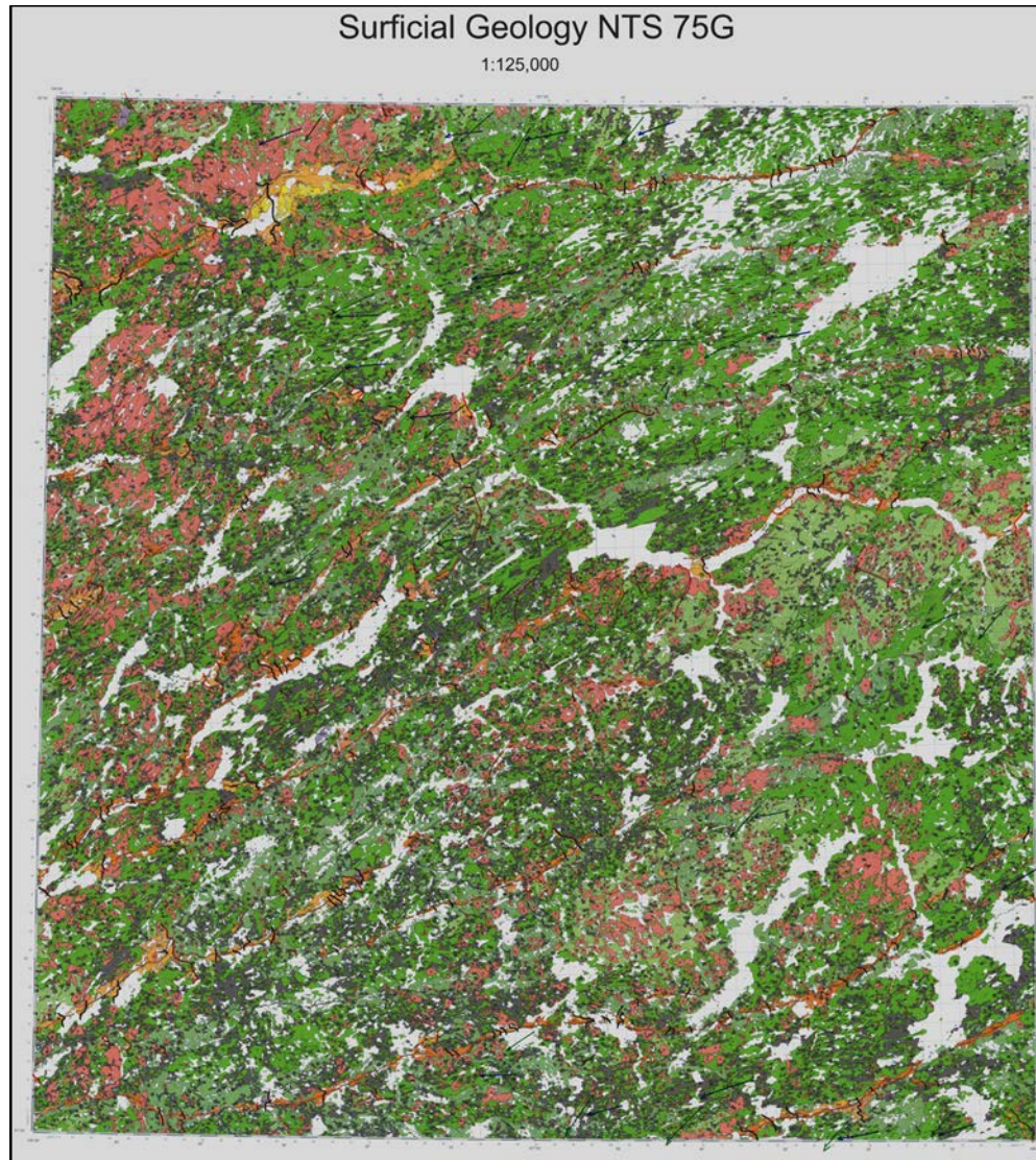
Figure 3. Surficial geological map for NTS 75G based on airphoto interpretation. This summer's mapping in 75G focused on ground-truthing the map and key questions that arose from the preliminary interpretation.
