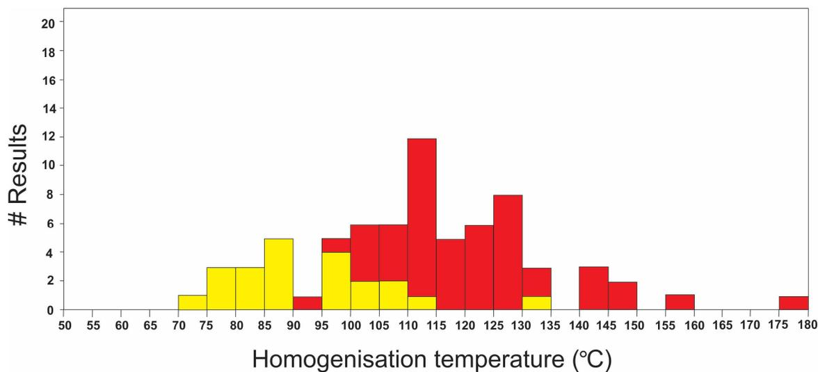
Figure 6. Histogram showing the distribution of fluid inclusions homogenization temperature ( $T_h$ ). Late calcite cements are in yellow and recrystallized early marine cements are in red.
