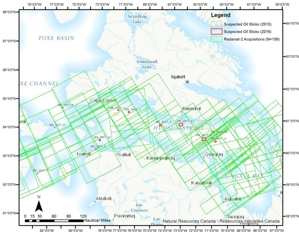
Figure 9. The green rectangles in the figure below show the distribution of the image footprints for 2016. There are 109 images in total (VV polarization, 12.5 m pixel spacing). The suspected oil slicks for 2016 are indicated with red boxes
