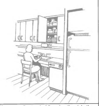
If you usually stand while using the sink, the sink should be at a height requiring minimal bending. If you wish to sit while using the sink, there should be space under the sink for knees and the sink should be at a height requiring minimal stretching.
