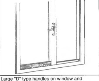
Large "D" type handles on window and extension arm on window lock are easier to grip for people with decreased strength and movement in the hand.
