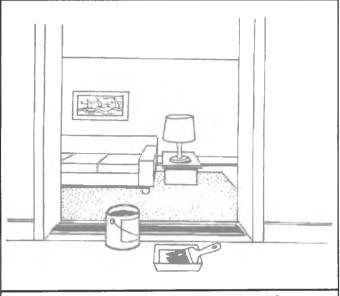
Strong colour contrast strip on edge of step or threshold or changes in floor texture between rooms, will help people with poor vision detect possible obstacles.
