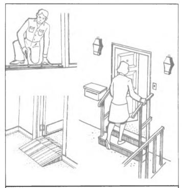
A flat threshold with a soft vinyl strip in the centre, a small ramp or an extra step with a grab bar or handrails are possible solutions for dealing with high door thresholds.
