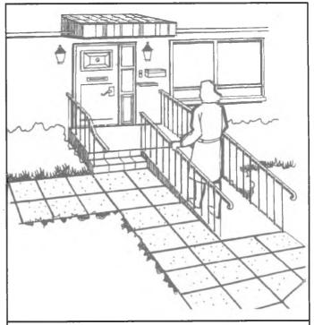
A ramp next to existing steps gives the option to a person with a walker or a wheelchair. Handrails along the entranceway guide and support persons with poor vision or balance.
