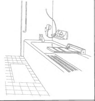
When using a shower seat, a hand held shower, mounted on a vertical rod or on a low bracket makes washing and rinsing easier.
