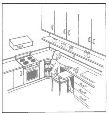
Pull-out shelves are ideal to allow food preparation in a seated position. "U" or "L" shaped counters, cut down the amount of necessary walking.
