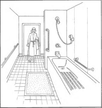
A vertical grab bar at tub entrance gives a first support while the horizontal grab bar along wall will help you complete the entrance and lower yourself onto shower seat or to bottom of tub.
