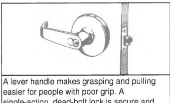
single-action, dead-bolt lock is secure and only requires the use of one hand.
