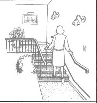
Well lighted staircase with solid handrails extending beyond the top and bottom of stairs, strong colour contrast or changes in texture at the top or bottom make it safer and easier for people with poor balance or people with poor vision. 3.1 Do you have any difficulty moving from one room to another?
