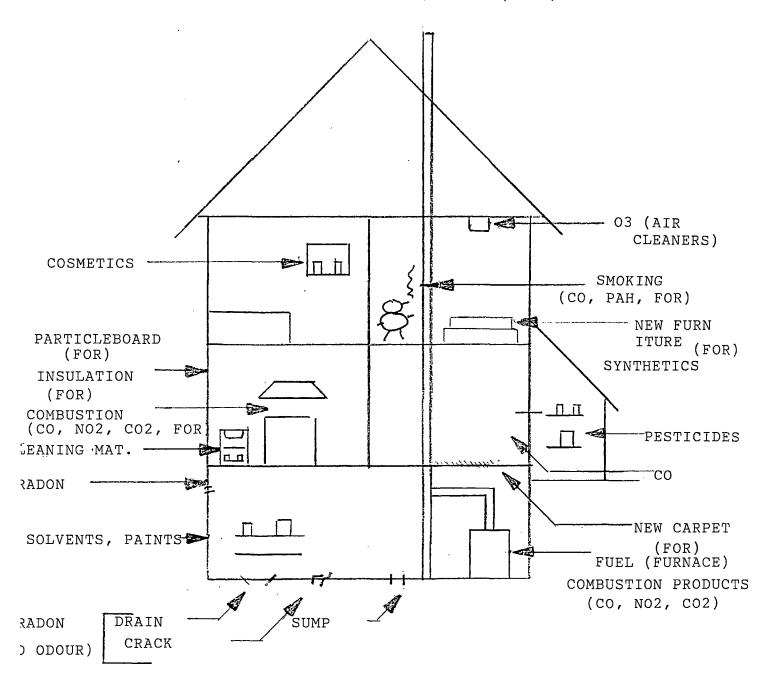
ODOURS MOVE FROM SOURCE BY MEANS OF PATHWAYS (DOORS, VENTILATION)
