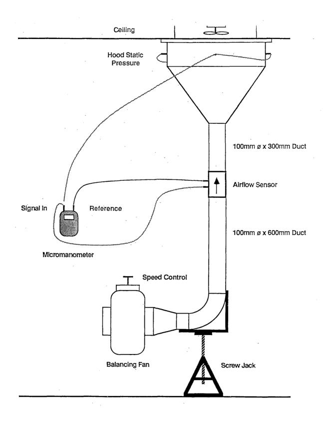
Figure B. Bathroom Exhaust Fan Airflow Test Set-up
