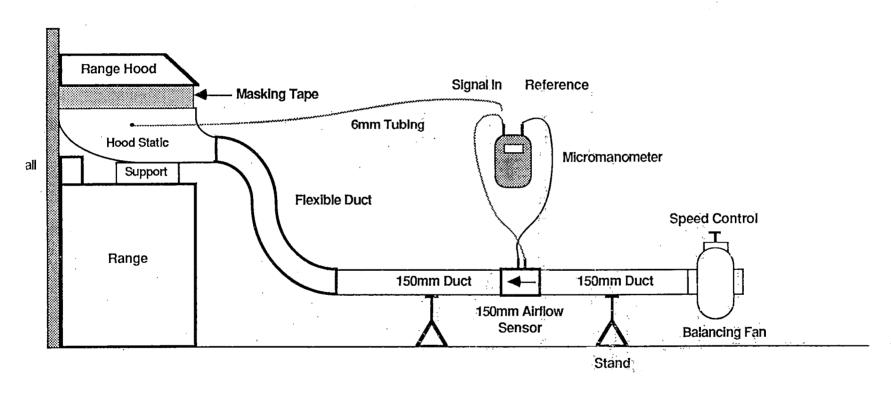
Figure A: Range Hood Airflow Test Set-up
