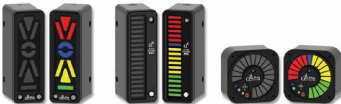
Example of some AOA indicators that could be viewed in a cockpit. The color ranges indicate the available lift reserve: green is normal, yellow indicates a gradual reduction in lift (the pilot is pulling too hard), and red indicates approaching the critical angle of attack (the wing is about to stall).
