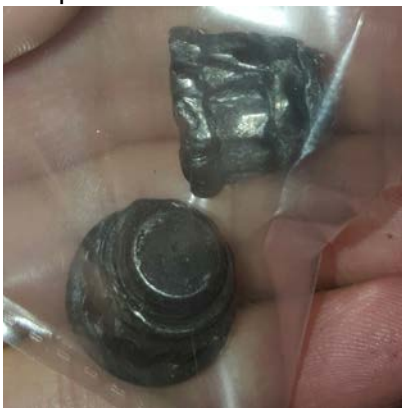
Sheared nuts from main wheel tie bolts
