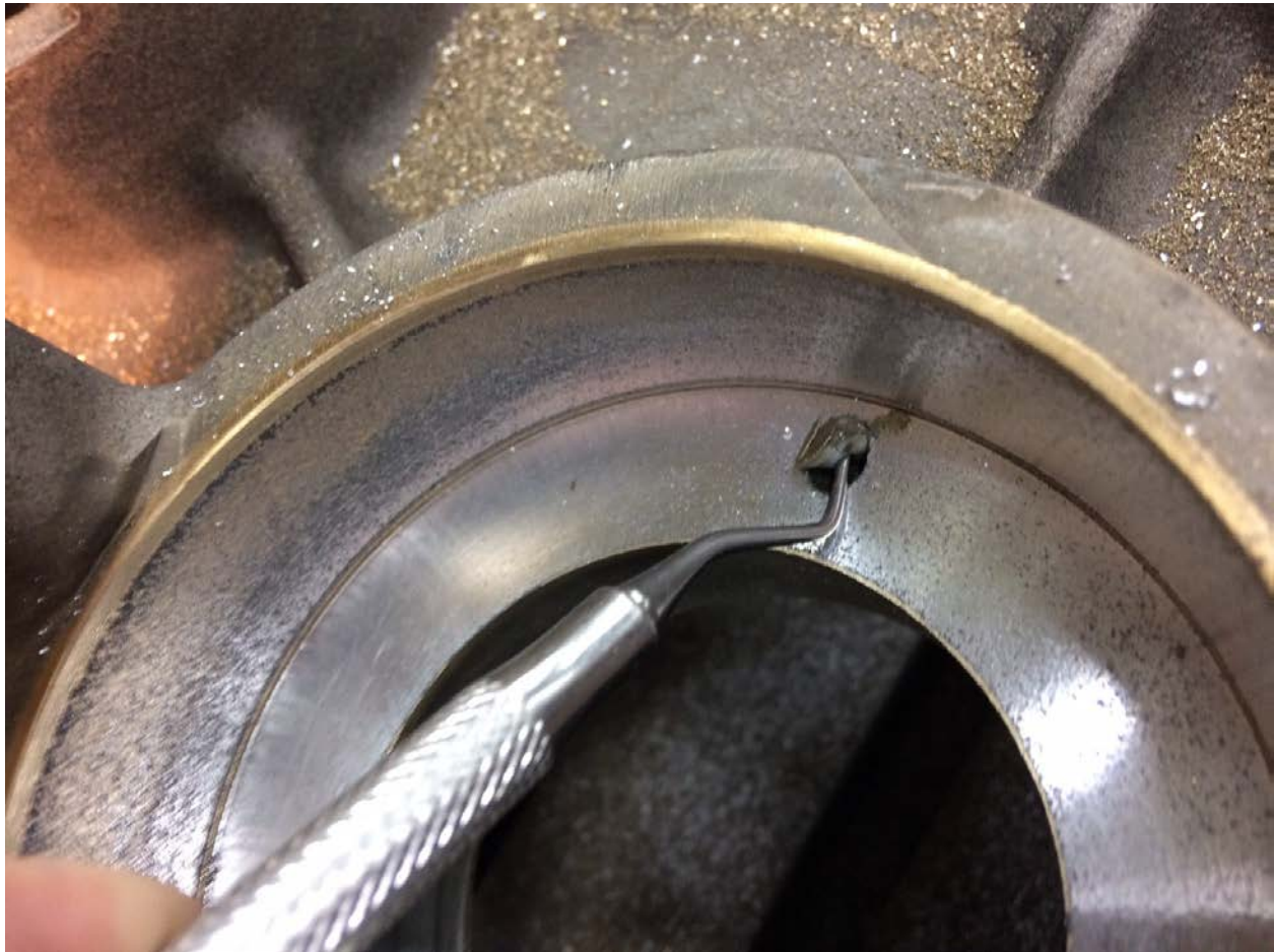
Bearing cavity with rubber plug left after previous repair
