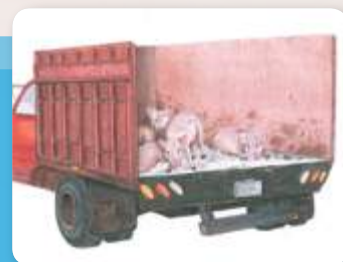
Inappropriate (e.g. unsecured load, improper footing, exposure to weather, etc.)
