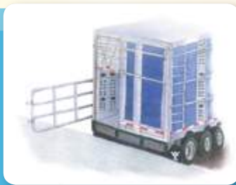
Configuration of unsuitable loading facility (e.g. gap, no ramp)
