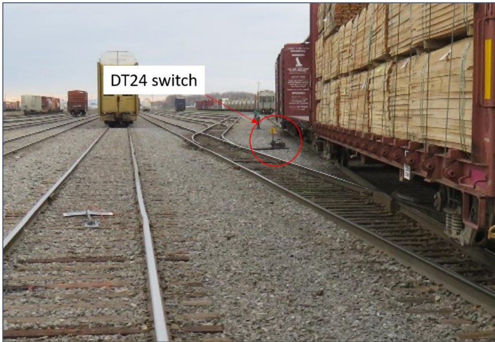
Figure 6. DT24 switch in the reverse position (Source: TSB)
