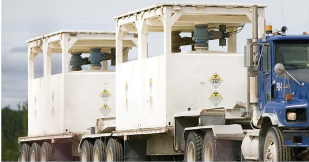
Figure 6.2: Ore slurry being transported from McArthur River to the Key Lake mill
