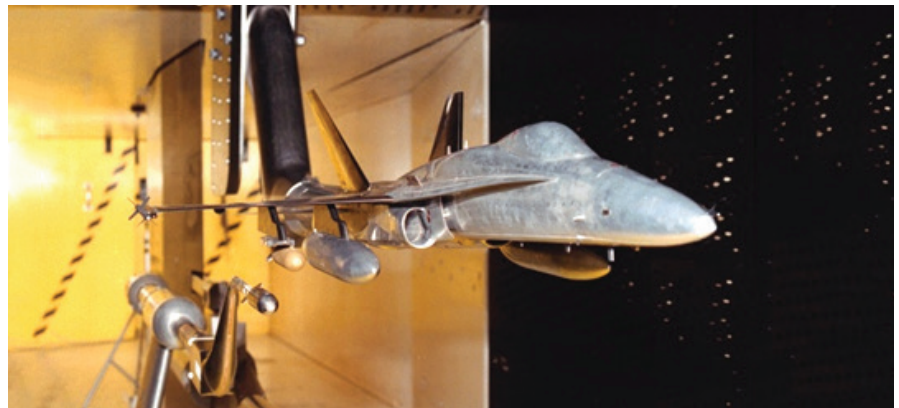
CF-18 on roof-mounted sting during stores release test.
