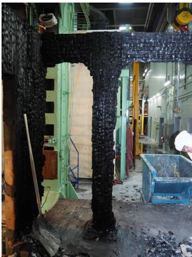
(c) Glulam beam and column
