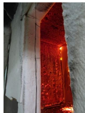
(b) CLT room at 120 min
