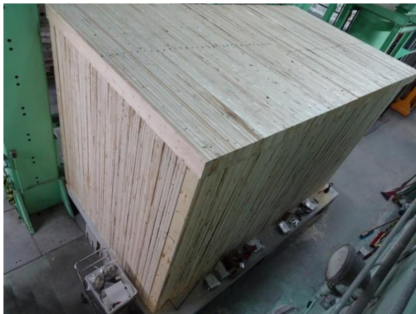
(c) outside view of NLT ceiling, Walls A and B
