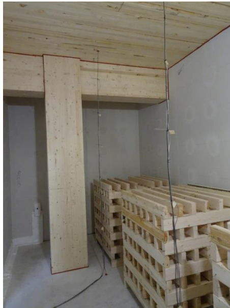
Figure 14. Fully exposed NLT ceiling, Glulam beam and column for Test NLT-1.
