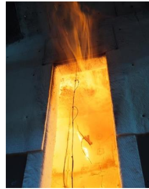
(b) CLT room at 240 min
