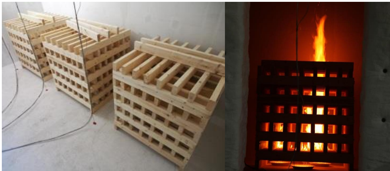
Figure 8. Photographs of (a) wood cribs and (b) middle crib ignition.
