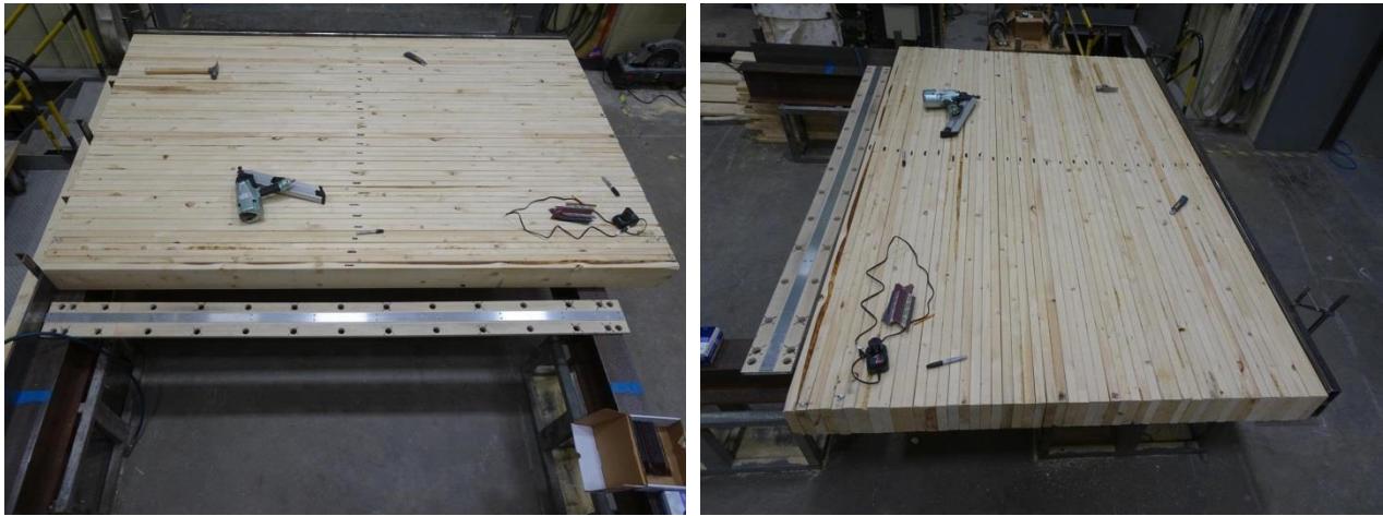
Figure 1. Photographs of NLT panel fabrication.
