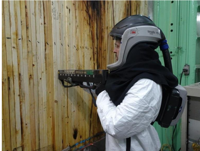
Figure 22. A Resistograph drill used to determine NLT char depth after the test.
