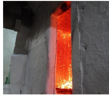
(b) Wall D and ceiling at 60 min
