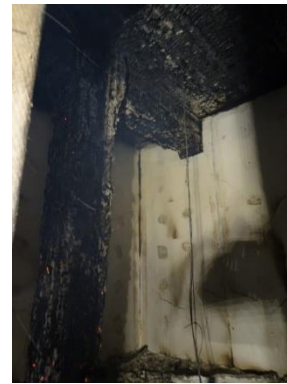
(b) CLT room at 220 min
