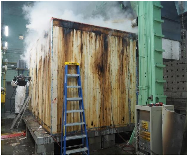
(a) NLT exterior (gypsum board removed)
