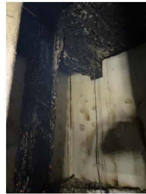
(b) CLT room at 220 min
