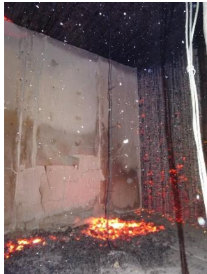
(c) Wall A (partial), Wall B and ceiling at 90 min
