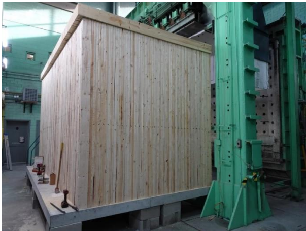
(a) outside view of NLT Walls A and D
