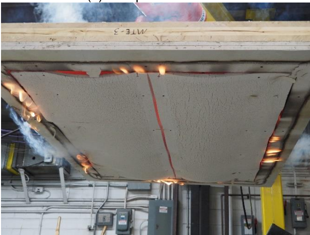
(c) gypsum board stayed during test
