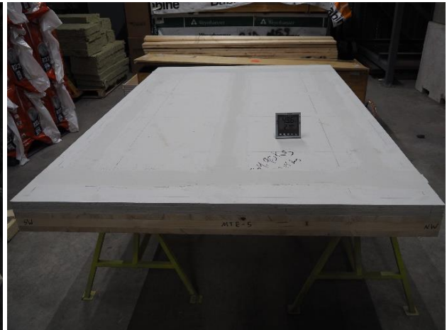
(b) encapsulated underside to fire exposure
