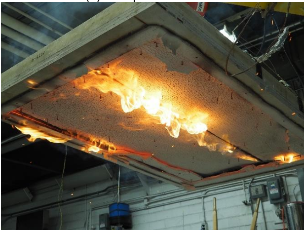
(c) gypsum board face and mid layers lost
