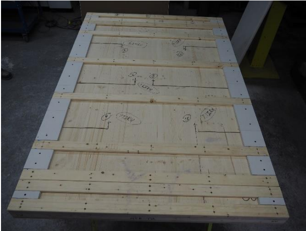
(a) wood furring on CLT underside
