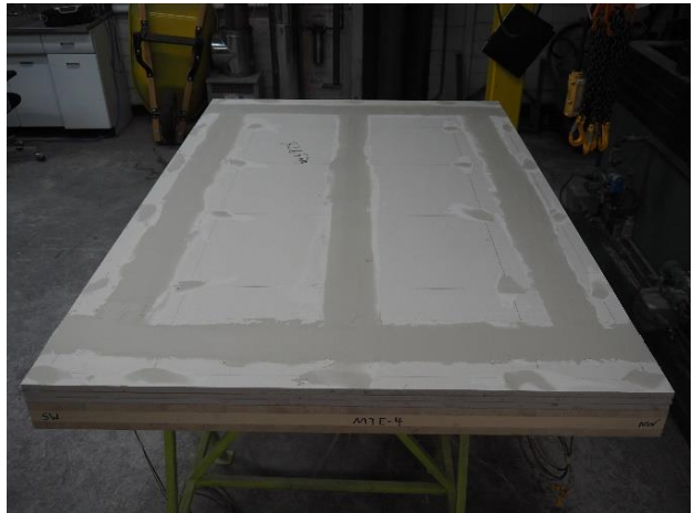
(b) encapsulated underside to fire exposure
