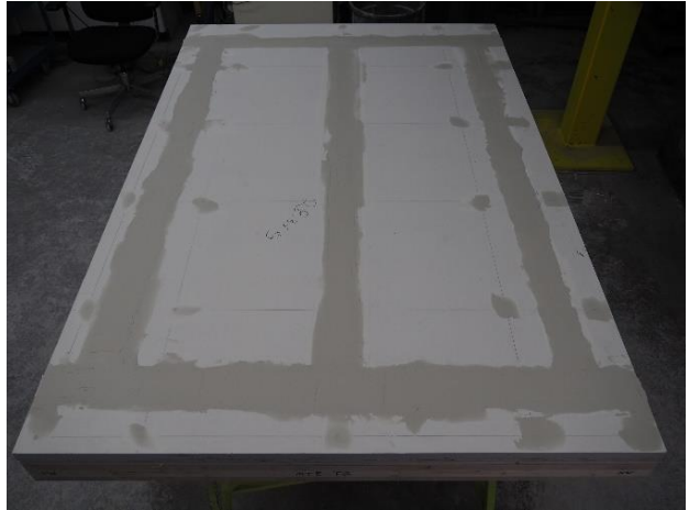
(b) encapsulated underside to fire exposure
