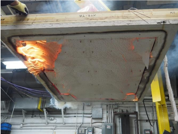
(c) face layer and partial mid layer of GB lost
