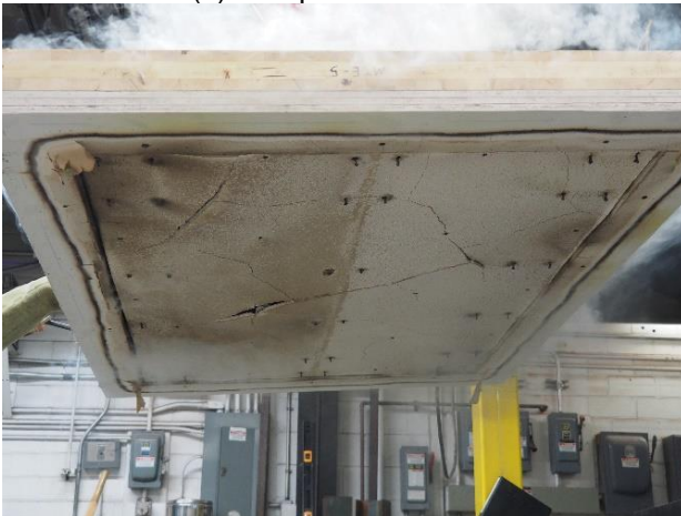
(c) gypsum board face layer lost
