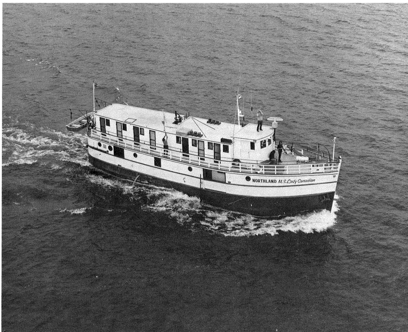
FIG. 15. The Lady Canadian , a charter vessel used for Lake Winnipeg surveys. In spite of its elderly appearance, this vessel was filled with the latest INDAPS automated equipment. (Note the outboard transducer strut.)
