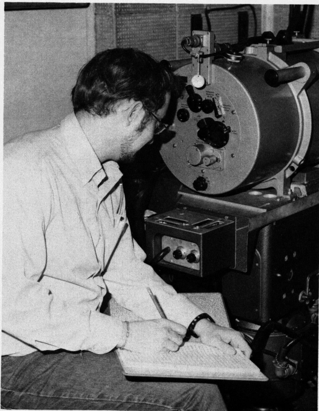
FIG. 18. Askania gravity meter used on multiparameter offshore survey.
