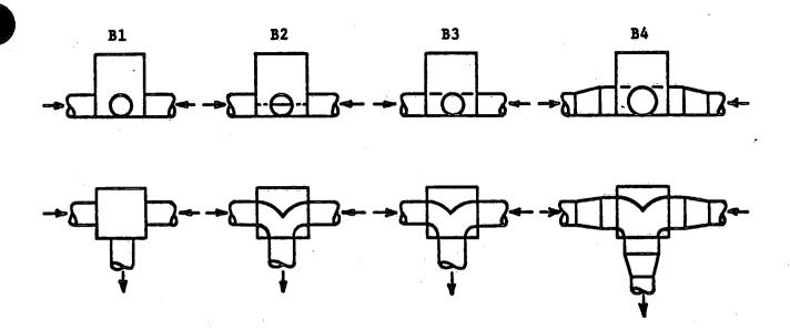
Fig. 2. Benching Designs Tested
