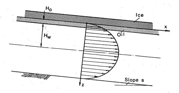
Fig. 1. The movement of a continuous oil slick.
