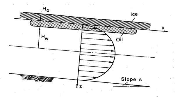
Fig. 2. The movement of a large oil patch.
