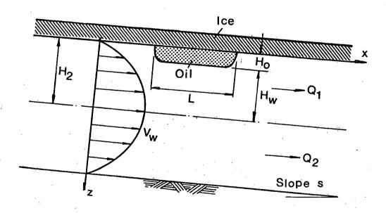
Fig. 3. The movement of an oil pocket of finite size.
