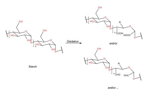
Oxidized Starch (~ 1.5% w/w) R = CH<sub>2</sub>OH or COOH
