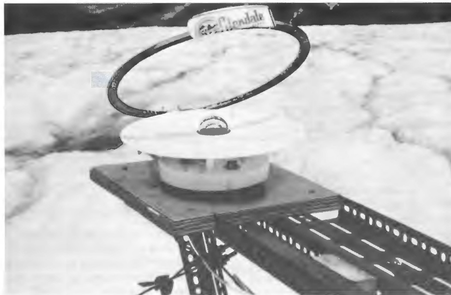
Figure 3. Kipp and Zonen pyranometer measuring diffuse radiation only.
