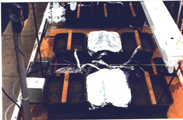
Figure 5-1(a). Experimental setup for greenhouse duckweed culture consisting of six experimental units. Aluminum foil covers the two duckweed-free controls and the influent delivery tubes, to prevent algal growth. Multi-channel peristaltic pump is at lower right. Influent reservoir (white) and effluent storage container (blue) are just visible behind rows of tubs. One lamp housing has been removed to allow photography.
