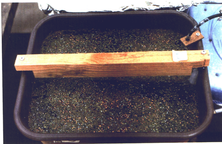
Figure 5-1(b). Detail of duckweed culture unit. Wooden brace supports transparent acrylic plastic baffle. Inlet is at upper right and outlet (not visible) is underwater at lower right.
