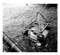
The oil is pumped out of the collection chamber. It is then either treated by gravity separation and/or recovered directly, depending upon the amount of entrained water.
