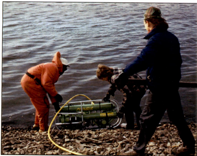
Figure 8: Remotely operated vehicle used to survey study sites
