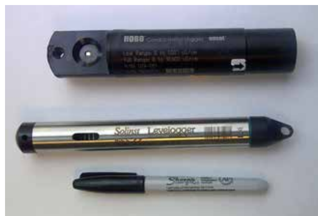
FIGURE A2. HOB0® U24 (top) and Solinst LTC Levelogger® (centre). Photo by Patrick Shaw.
