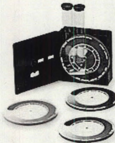
Figure 4-2: DPD Colour Disc (Hach)
