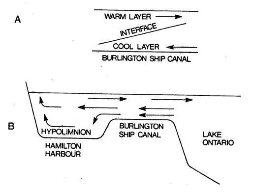
Fig. 1 Simplified models for water exchange between Hamilton Harbour and western Lake Ontario. A- Dick and Marsalek's (1973) model; B-Klapwijk and Snodgrass's (1985) model.
