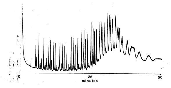
Figure 2. Gas Chromatogram of Dobanol 25-9 Surfactant. Conditions are given in text. Temperature programmed from 70 °C to 280 °C @ 5 °C/min and hold for 10 minutes.
