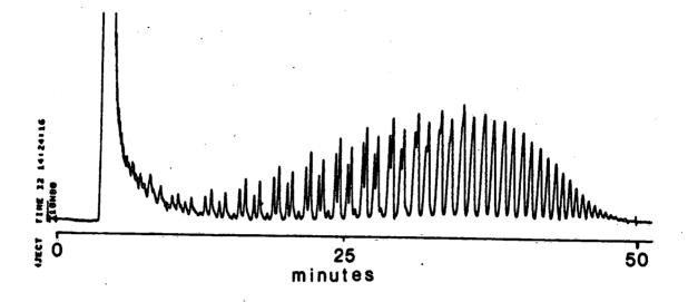
Figure 1. Supercritical Fluid Chromatogram of Dobanol 25-9 Surfactant.
