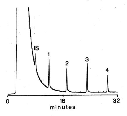
Figure 4. Supercritical Fluid Chromatogram of HBr Cleaved Dobanol 25-9.
