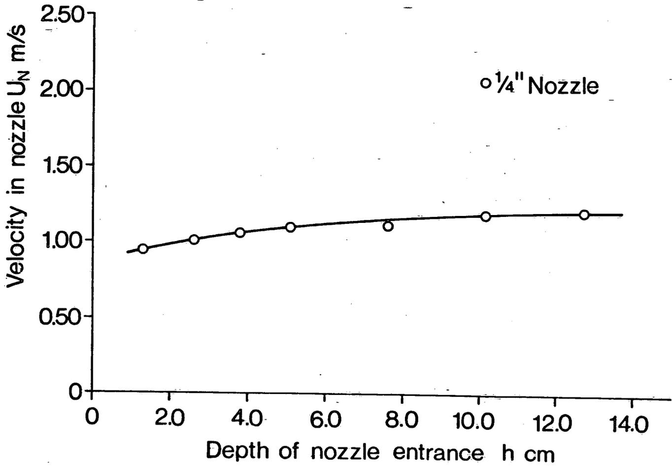
Figure 4 Calibration Curve for  $\frac{1}{4}$ " Nozzle obtained in WSC Constant Head Tank
