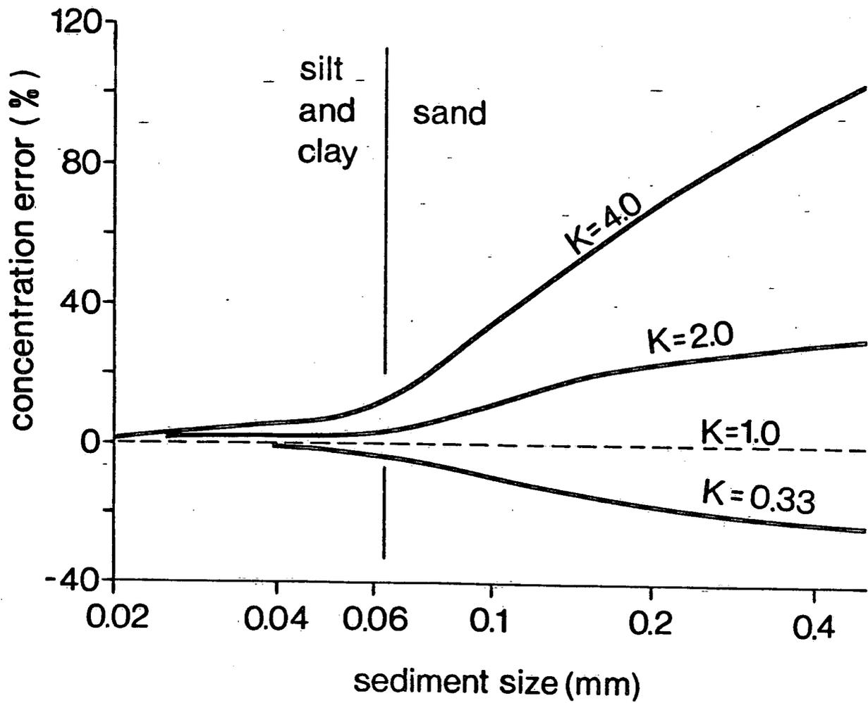
Figure 6 Errors due to over and under sampling (from Guy and Norman, 1970)
