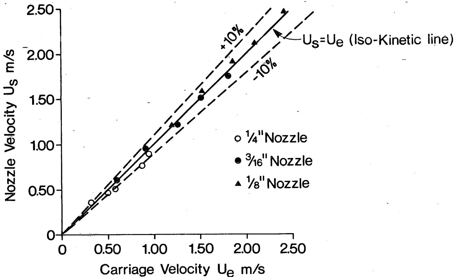
Figure 2 WSC Calibration for DH48 Sampler with three standard nozzles.
