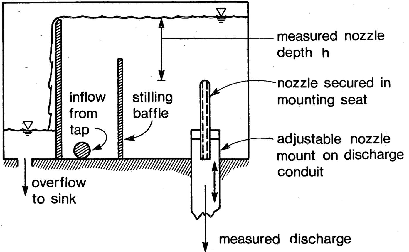
Figure 3 Schematic of WSC Constant Head Tank
