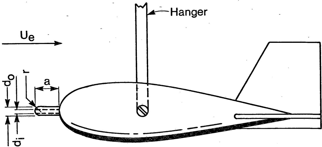
Figure 1 Schematic of Sampler and Nozzle
