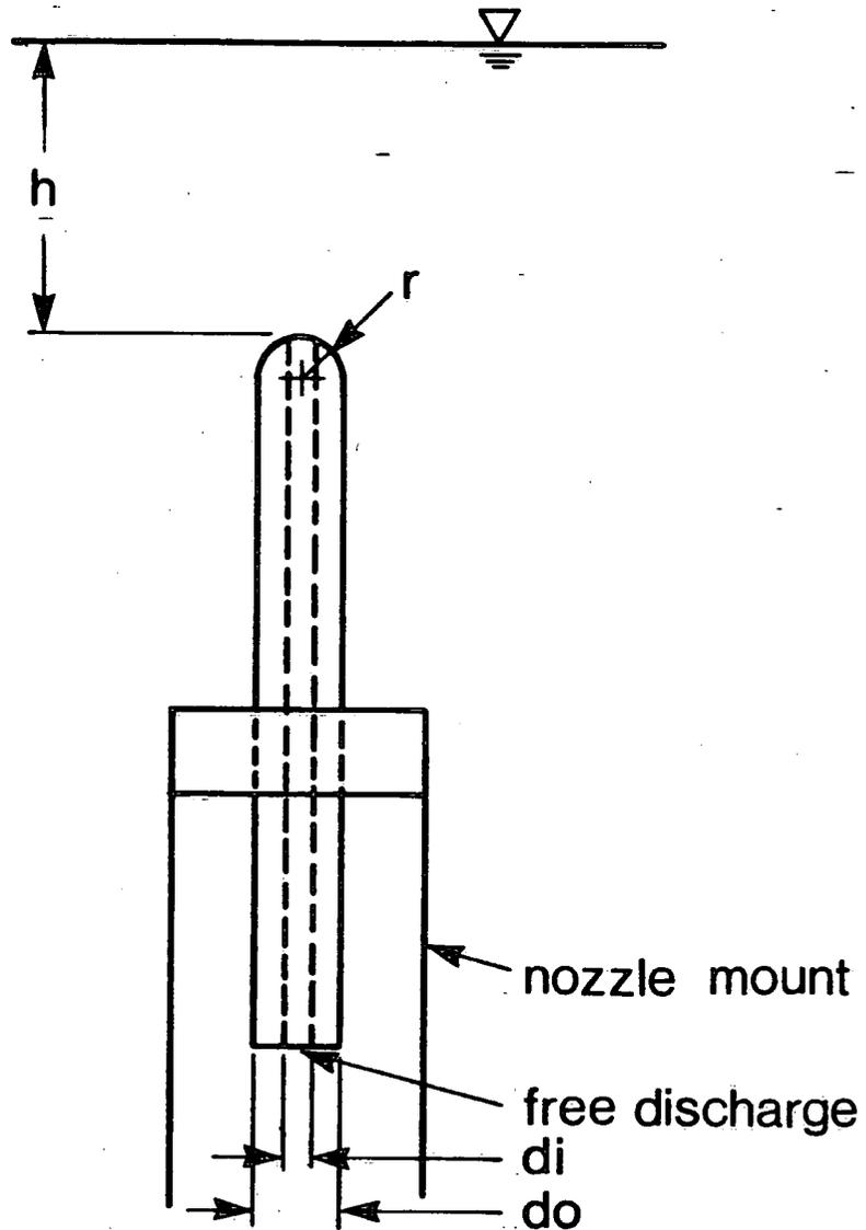
Figure 7 Schematic of Geometric Variables for Calibration of nozzle in WSC Constant Head Tank.
