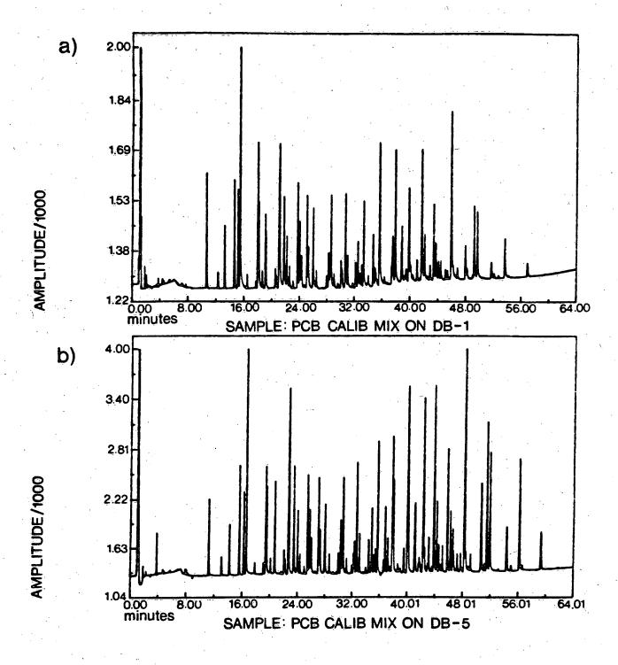
FIGURE 1. Dual Column Chromatograms of Calibration Mixture
