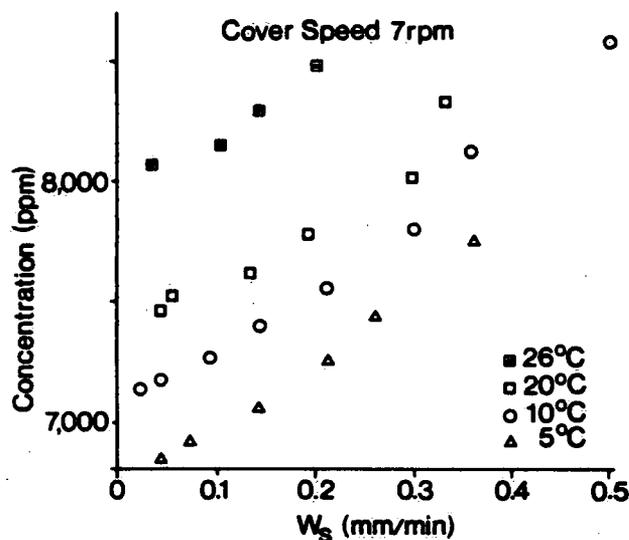
Fig 4. Temperature Effect on Settling Velocity-Concentration Curve
