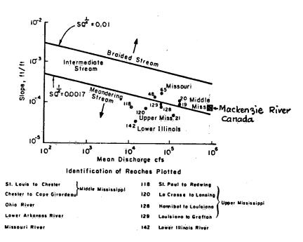
Fig. A. Slope-Discharge Relation for Braiding or Meandering in Sand Bed Streams (after Lane (1957))
