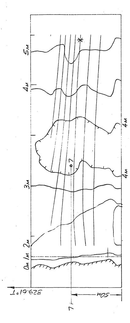
Wave rays at Van Wagner's Beach: wave parameters at the wave gauge array (\*) are given in Table 1; the sled-way is marked 7-7; the depth contours are relative to a datum of 74.8 m a.s.l. Experiment 4-2. Figure 5
