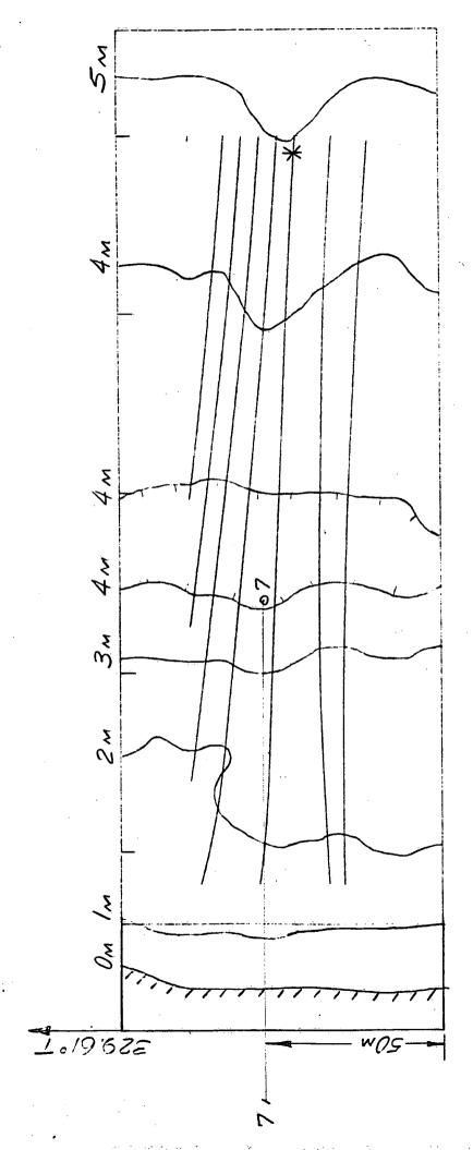
Wave rays at Van Wagner's Beach: wave parameters at the wave gauge array (\*) are given in Table 1; the sled-way is marked 7-7; the depth contours are relative to a datum of 74.8 m a.s.l. Experiment 16-1. Figure 13
