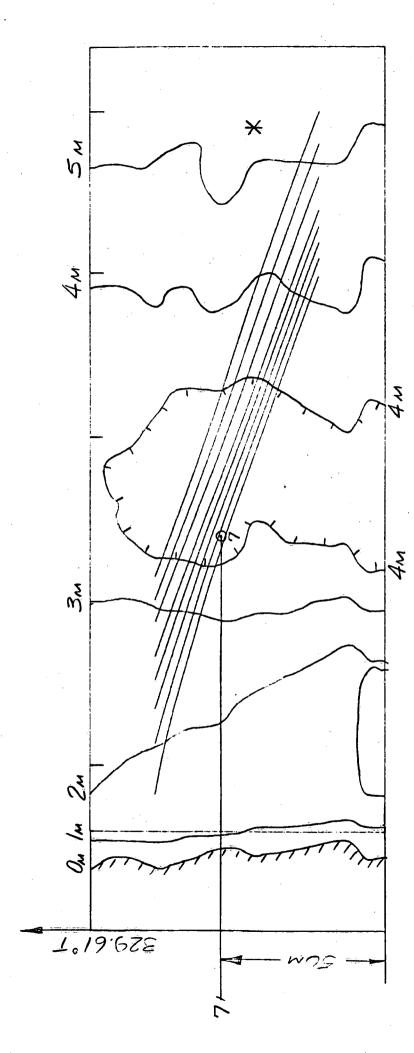
Wave rays at Van Wagner's Beach: wave parameters at the wave gauge array (\*) are given in Table 1; the sled-way is marked 7-7; the depth contours are relative to a datum of 74.8 m a.s.l. Experiment 4-1. Figure 4
