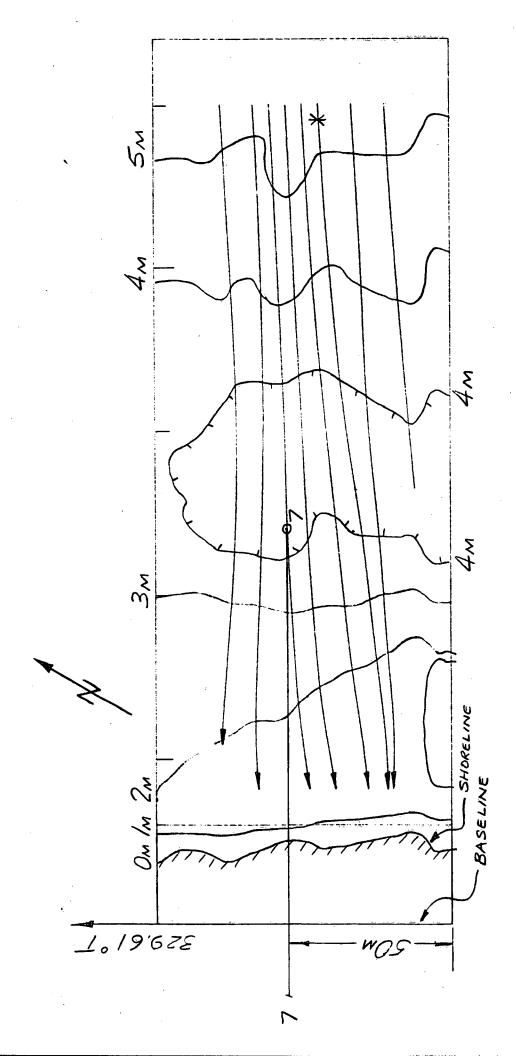
Wave rays at Van Wagner's Beach: wave parameters at the wave gauge array (\*) are given in Table 1; the sled-way is marked 7-7; the depth contours are relative to a datum of 74.8 m a.s.l. Experiment 2-2. Figure 1
