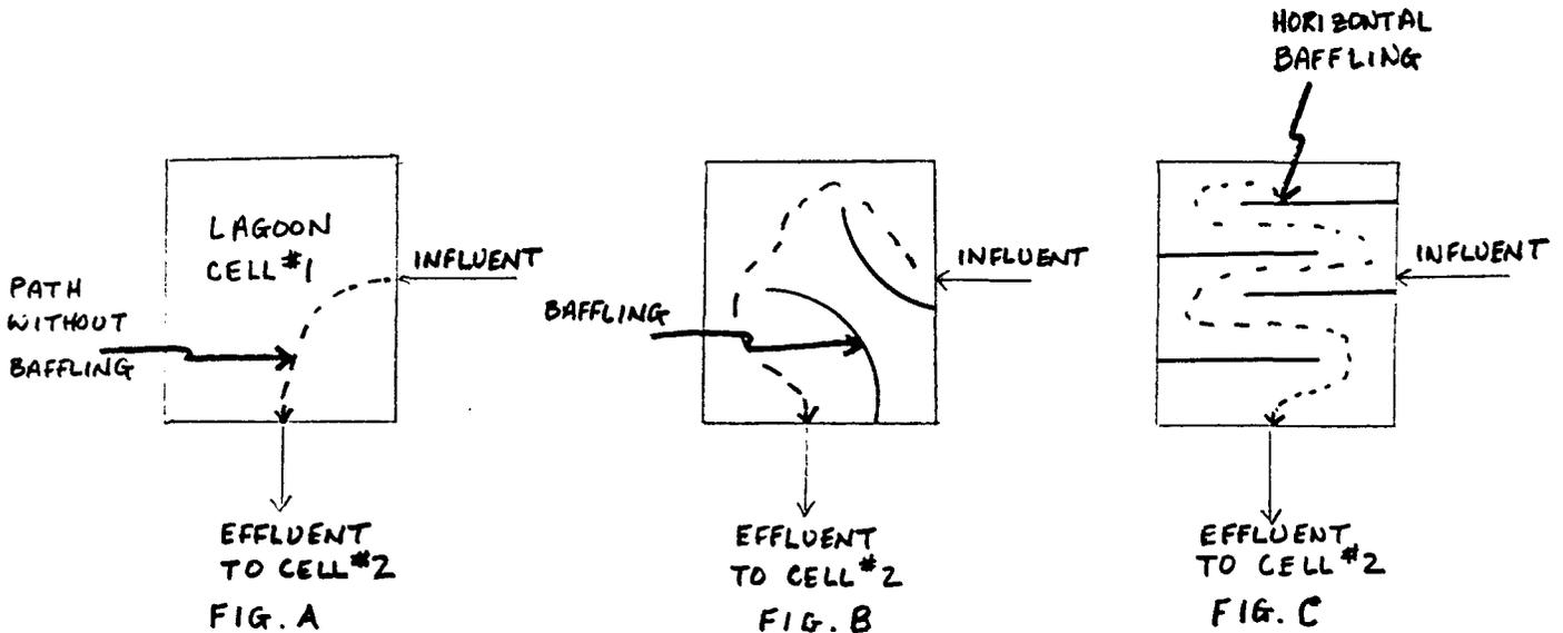
The incoming flow will proceed along a path of least resistance, that is, directly from inlet to outlet as outlined by the dotted lines in figure A. A configuration such as that shown in figures B or C would lower the degree of short-circuiting by ensuring greater distribution of flow throughout the cell before exiting through the outlet to cell #2. Although only suggestions, the addition of some baffling is worth considering in view of the high degree of short-circuiting in all cells.
