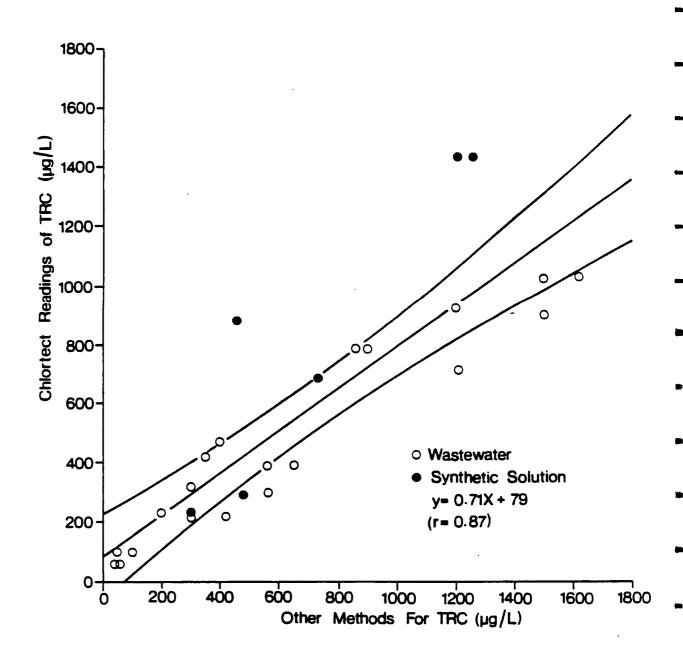
FIGURE 2A CORRELATION OF CHLORTECT READINGS VERSUS TOTAL RESIDUAL CHLORINE LEVELS BY OTHER METHODS
