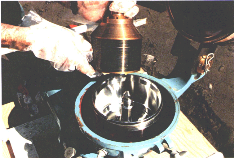
PLATE 7: Reinstalling distributor and dish assembly in bowl base.
