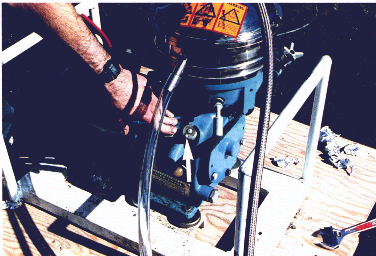
PLATE 23: Rotator shaft cover with dot to estimate centrifuge RPM.
