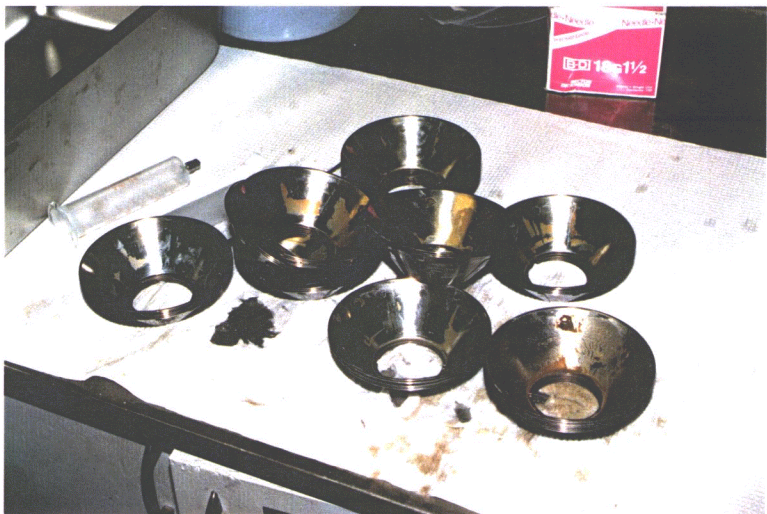
PLATE 28 : Fine sediment adhering to discs, from pulp mill sample.
