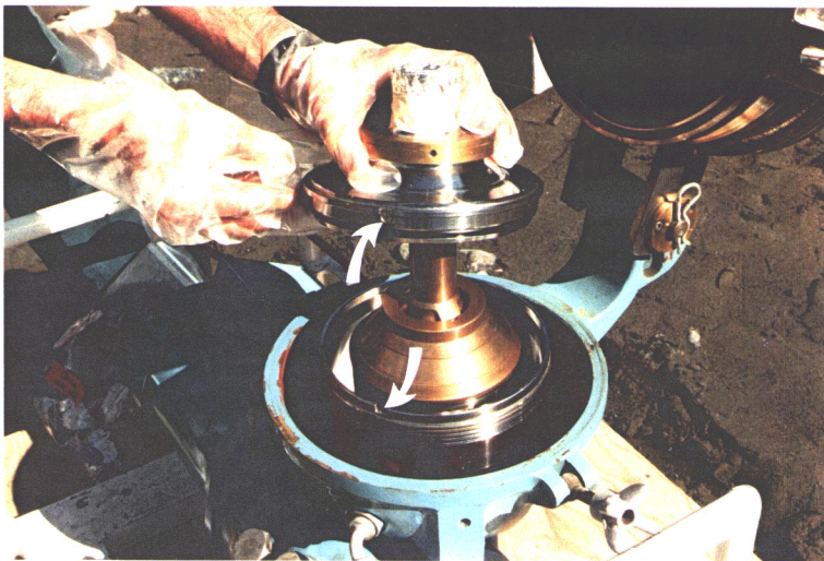
PLATE 8: Installing the bowl hood by lining up key in the hood with key slot in base.
