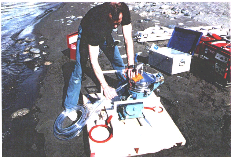
PLATE 13 : Installing thick-walled Tygon tubing to discharge pipe.
