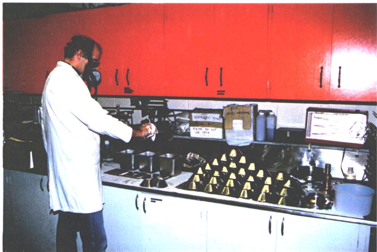
PLATE 29 : Solvent washing discs by sequential emersion in SS vats containing acetone, hexane, and dichloromethane.
