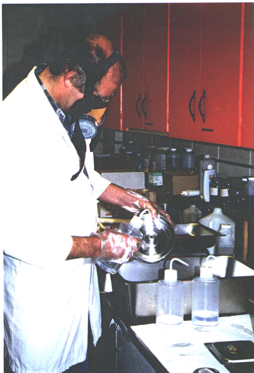
PLATE 30 : Solvent washing bowl parts using Teflon wash bottles, and wearing appropriate safety breathing apparatus when fume hood not available.
