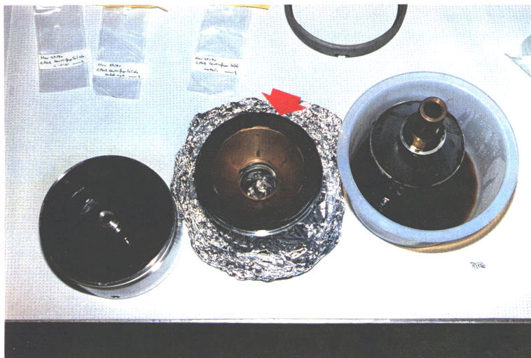
PLATE 24: Inverted bowl hood with sediment cake on rim, distributor assembly in Teflon basin and bowl with sediment sample.
