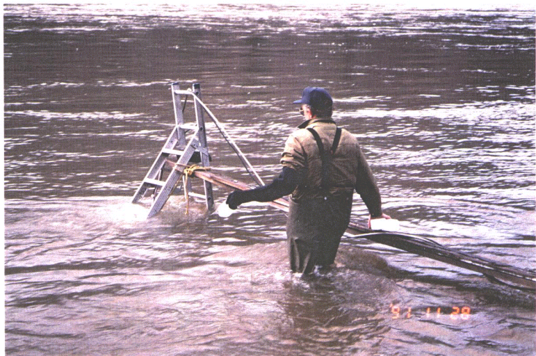
PLATE 19: Ladder (tripod) set-up supported by plank connected to shoreline. Hoses and electrical cords run along plank out of water for safety.
