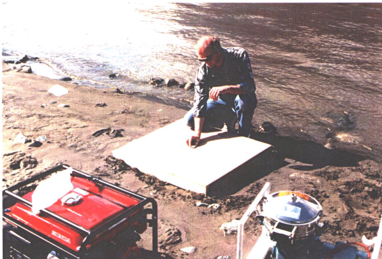
PLATE 4: Levelling a pallet for centrifuge platform.
