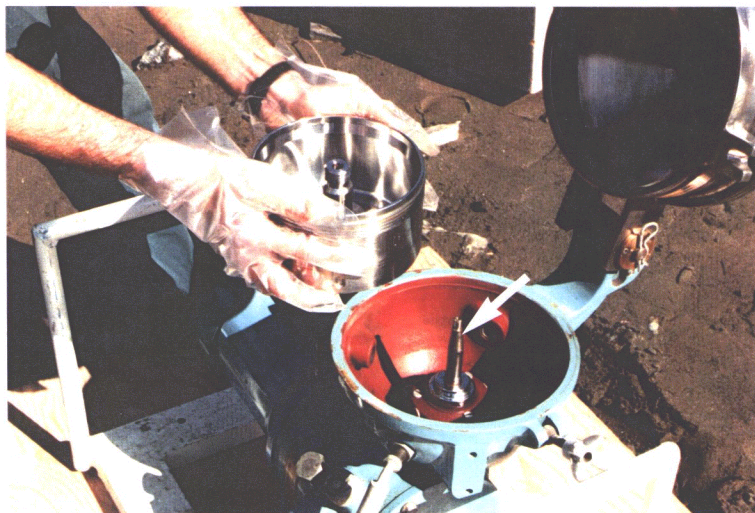
PLATE 5: Installing bowl base on centrifuge spindle.
