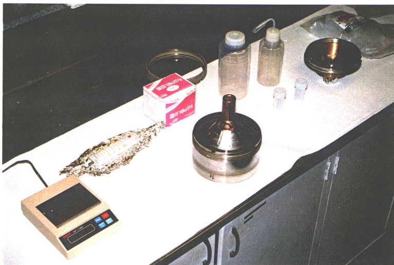
PLATE 26: Equipment for sample retrieval including glass 50 mm syringe, Teflon sample bottle for bowl liquid, and Teflon wash bottles in a clean work area.
