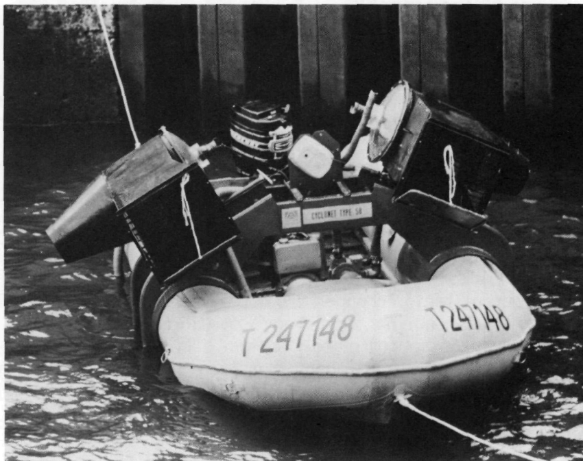
Plate 2 - Cyclonet 050 System Mounted on ZODIAC (Package as originally received)
