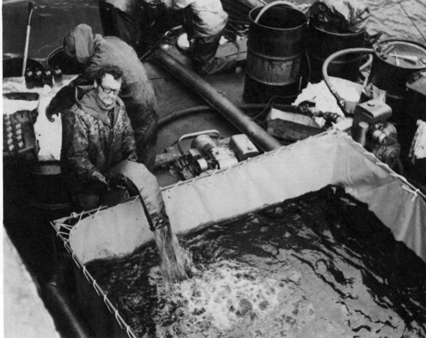
Plate 16 - Pumping Oil and Water from Watermaster into "Porta-Tank"
