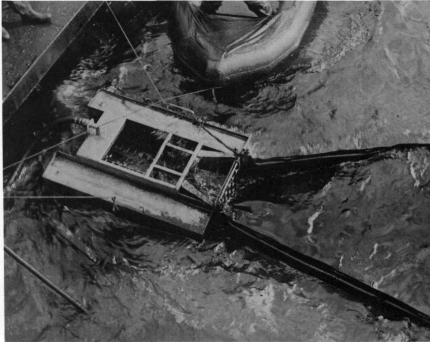
Plate 3 - MacMillan-Bloedel Skimmer in 30 cm Waves (Note oil escaping at boom connection)
