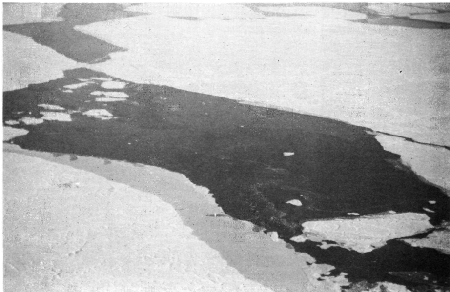
Plate 4 Open Crack Representing Next Stage in Deterioration From Conditions Above (Plate 3) Scale (picture centre) Approx. 1 cm = 80 m
